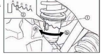
To decrease the spring preload, turn the adjusting ring in Direction (b).
