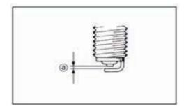
**NOTE**: Tightening torque of spark plug: 20N · m
